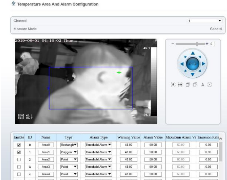
Figure 4-11 Temperature area and alarm configuration
