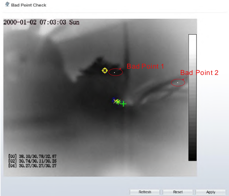
Figure 4-15 Bad Point Check
