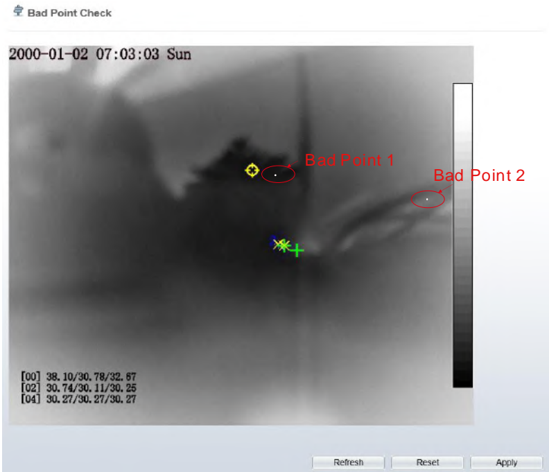
Figure 4-14 Bad Point Check
