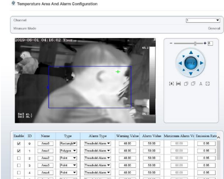
Figure 4-10 Temperature area and alarm configuration
